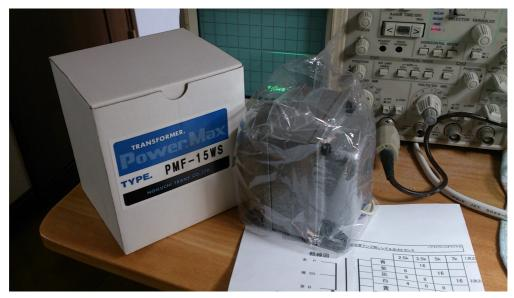
Noguchi Transformer PMF-15WS can be use for Single Ended Amplifier for 12A ,2A3 , WE275 , 300B VT52 , VT62 , 45 , KT88 and EL34 . Charactor is next figure.
